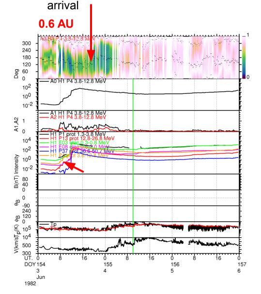
IMP 8 0.5-4 MeV; Near isotropic early in event, changing abruptly to strong anti-solar streaming, then becoming less anisotropic. Flow reversal close to shock passage
